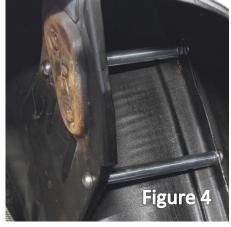
5. Locate and mark the torsion rod bracket and fender well lip for mounting of the support rods (figure 4). Drill holes accordingly, apply anti-seize to the threads and attach with stainless steel fasteners provided.
